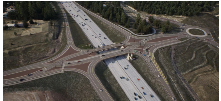
Graphic rendering of the new diverging diamond interchange design for the Interstate 25 and Happy Canyon Road interchange.
